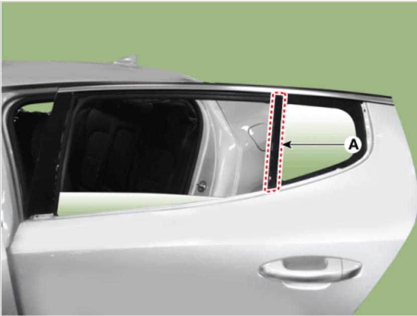
6. Remove the rear door frame molding (A) by using a remover.
