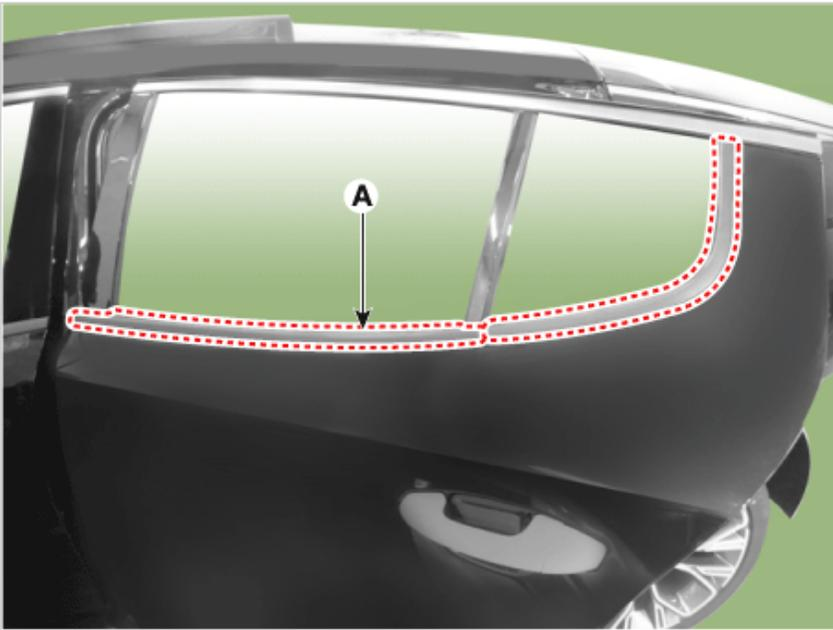
5. Remove the rear door drive channel (A) after loosening the mounting screws.
