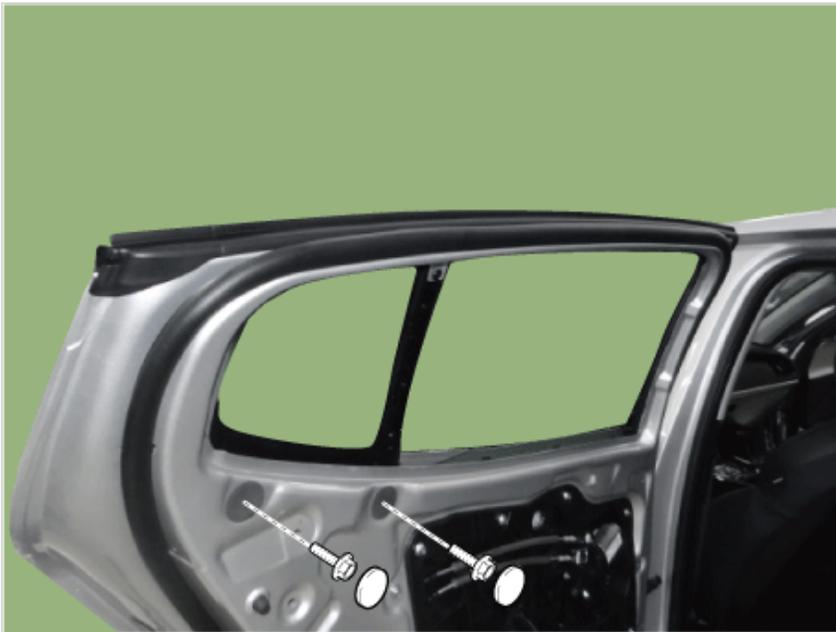
11. Remove the fixed glass (A) from the rear door panel.
