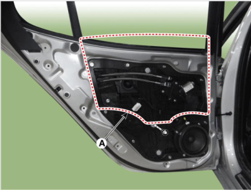
10. Remove the screen cap and then loosen the fixed glass mounting bolts.
