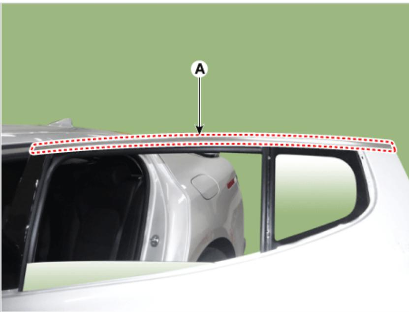
7. Remove the rear door frame garnish (A) and glass run.
