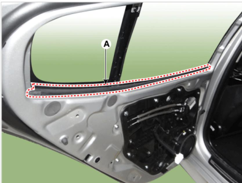
4. Remove the rear door belt outside weatherstrip (A) by using a remover.
